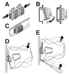
Figure 3 Mounting and removing
