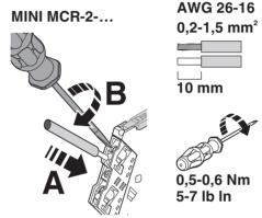
Figure 4 Screw connection
